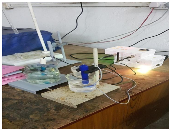
Fig. 2: IOT Sensor for water health monitoring
